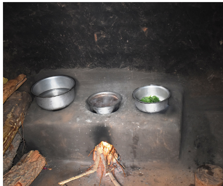
A cooking stove that uses less firewood with three places where one could be using for cooking
